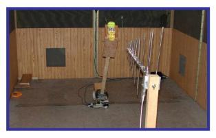
Test fixture for 40° measurements in RF screen room – McMurdo Fastfind Plus mounted
