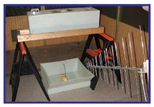
Test fixture for rain test
