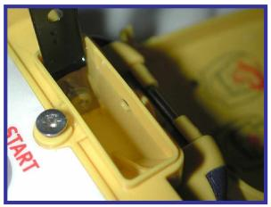
Water filled antenna storage well of McMurdo Fastfind Plus PLB
