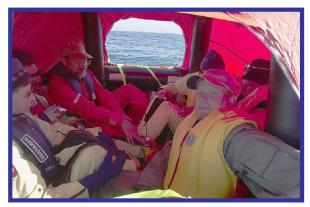
Maritime Scenario Delta – arrangement of life raft occupants in raft with McMurdo Precision EPIRB in center (typical) preparatory to starting testing.
