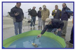
Maritime Scenario India – measuring 121.5 signal strength of McMurdo Fastfind Plus with base of the antenna submerged.
